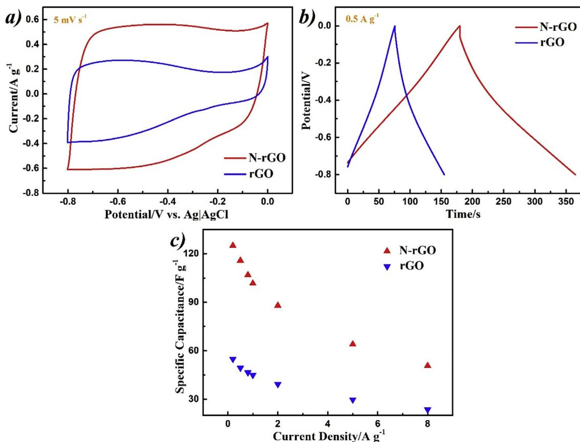
**Fig. 4.** Compared electrochemical performance of N-rGO and rGO in 6 M KOH. (a) CVs of N-rGO and rGO at a scan rate of 5 mV s<sup>-1</sup>; (b) galvanostatic charge/discharge curves of N-rGO and rGO at a current density of 0.5 A g<sup>-1</sup>; (c) specific capacitance calculated from the discharge curve for different electrodes at different scan rates. (A colour version of this figure can be viewed online.)
