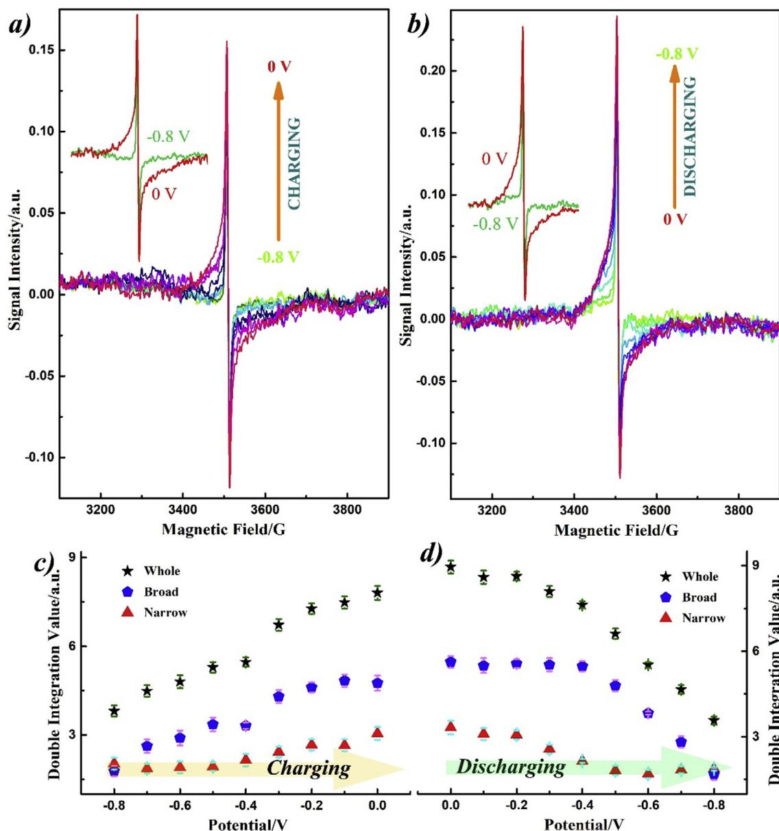
**Fig. 6.** *In situ* EPR spectra change of N-rGO over potential in 6 M KOH. EPR signal change under various potentials during charging (a) and discharging (b); the double integration value of each component during (c) charging and (d) discharging. Inner curves in (a) and (b) show the comparison of the NG electrode under 0 V and -0.8 V during charging and discharging. (A colour version of this figure can be viewed online.)
