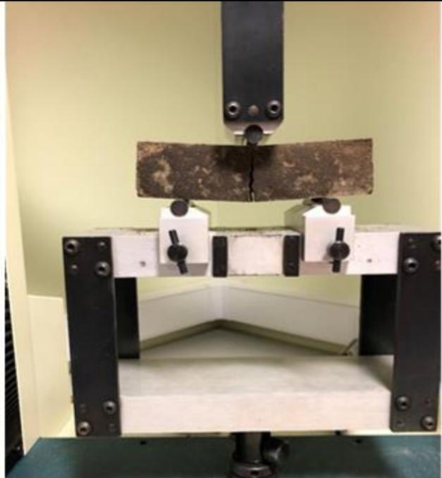
**Breaking the prism into halves**
