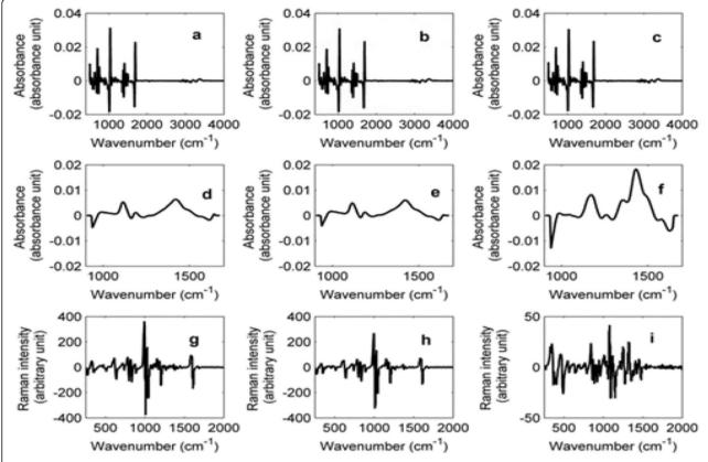
**Fig. 1** MSCD1 treated (**a**) FTIR spectrum modafinil tablets. **b** FTIR spectrum of pure modafinil. **c** FTIR spectrum lactose monohydrate. **d** NIR spectrum modafinil tablets. **e** NIR spectrum of pure modafinil. **f** NIR spectrum lactose monohydrate. **g** Raman spectrum modafinil tablets. **h** Raman spectrum of pure modafinil. **i** Raman spectrum lactose monohydrate measured using the Bruker Alpha FTIR, JDSU microNIR and Rigaku handheld Raman instruments, respectively
