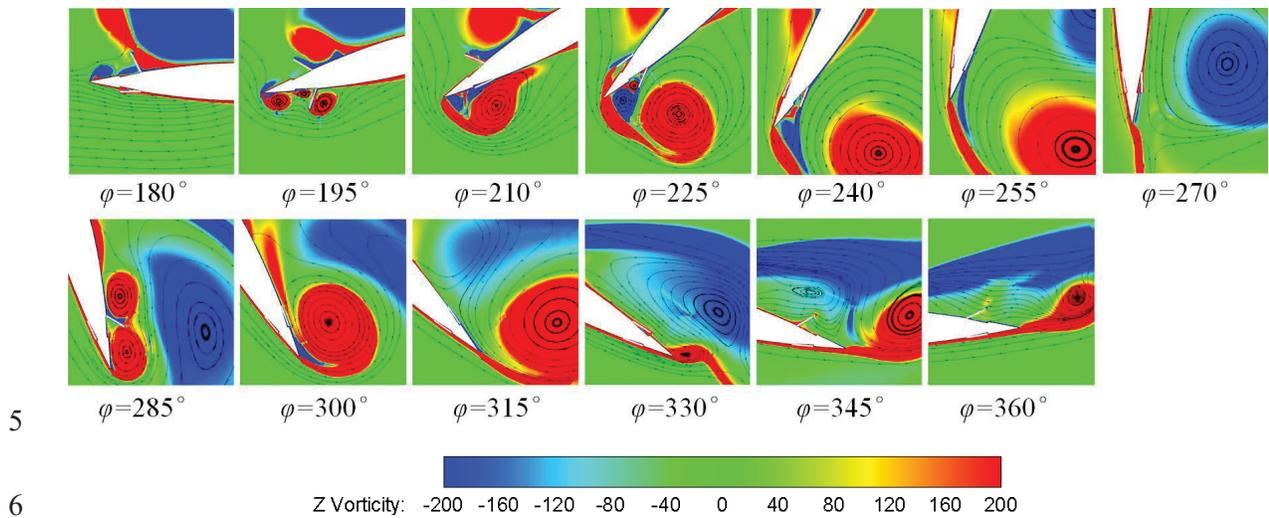
Fig. 21. Flow field around the outer flap at a TSR of 0.6
