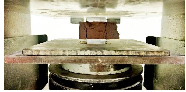
Fig. 7. Compressive strength test: (a) schematic and (b) experimental.
