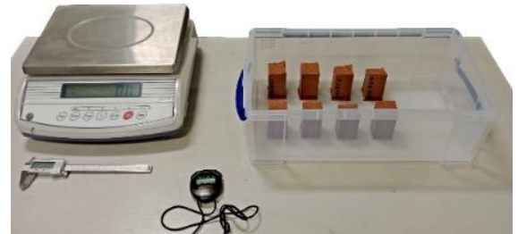
Fig. 8. Capillary water absorption test: (a) schematic and (b) experimental.
