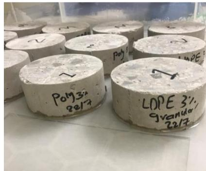
Figure 7 – Water absorption concrete via capillary.
