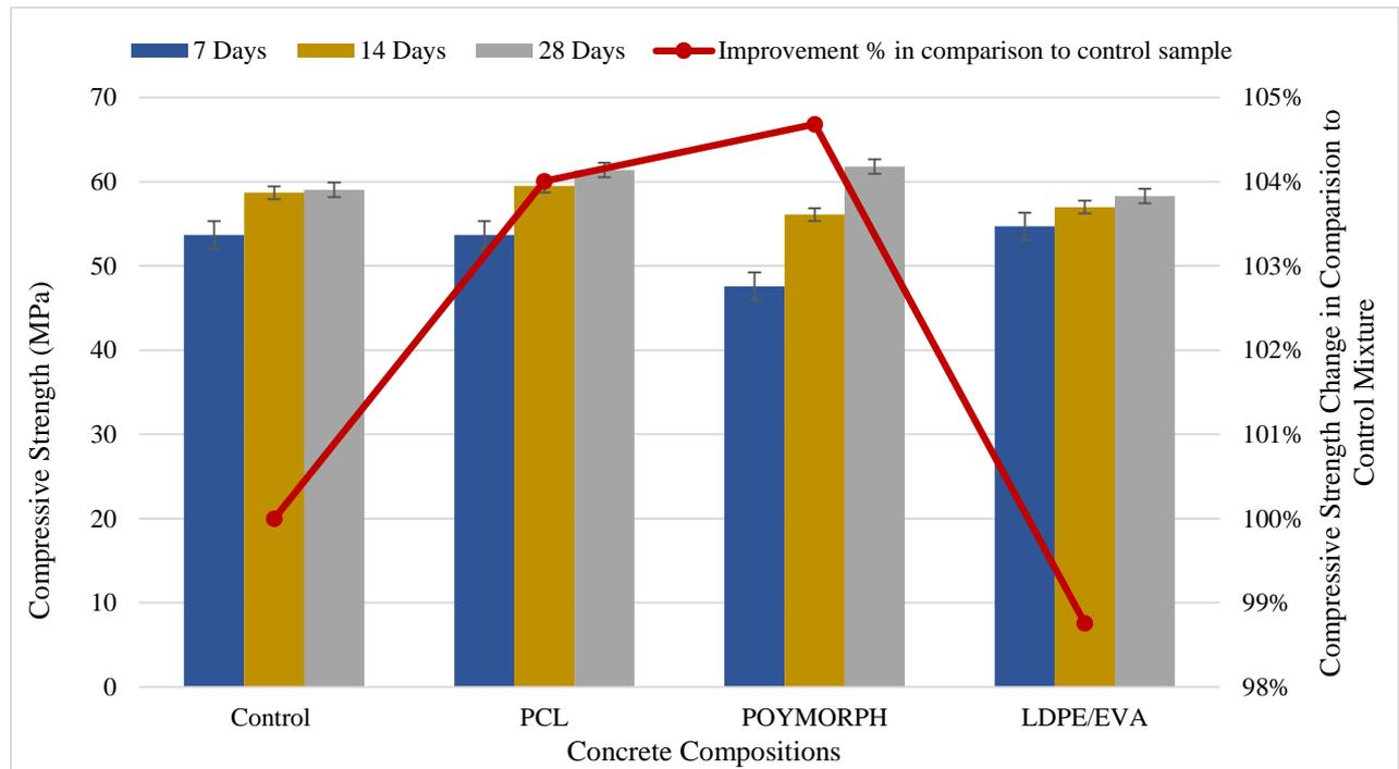
Figure 13 – Fine aggregate replacement by 3% granular thermoplastic polymer.
