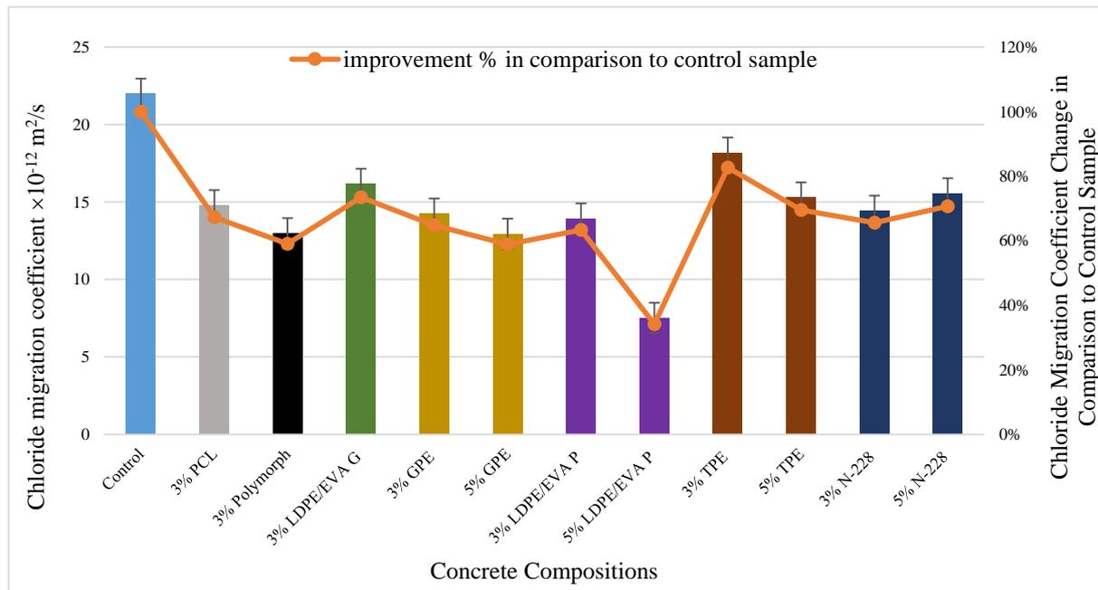
**Figure 20 – Coefficient of migration of all concrete compositions.**
