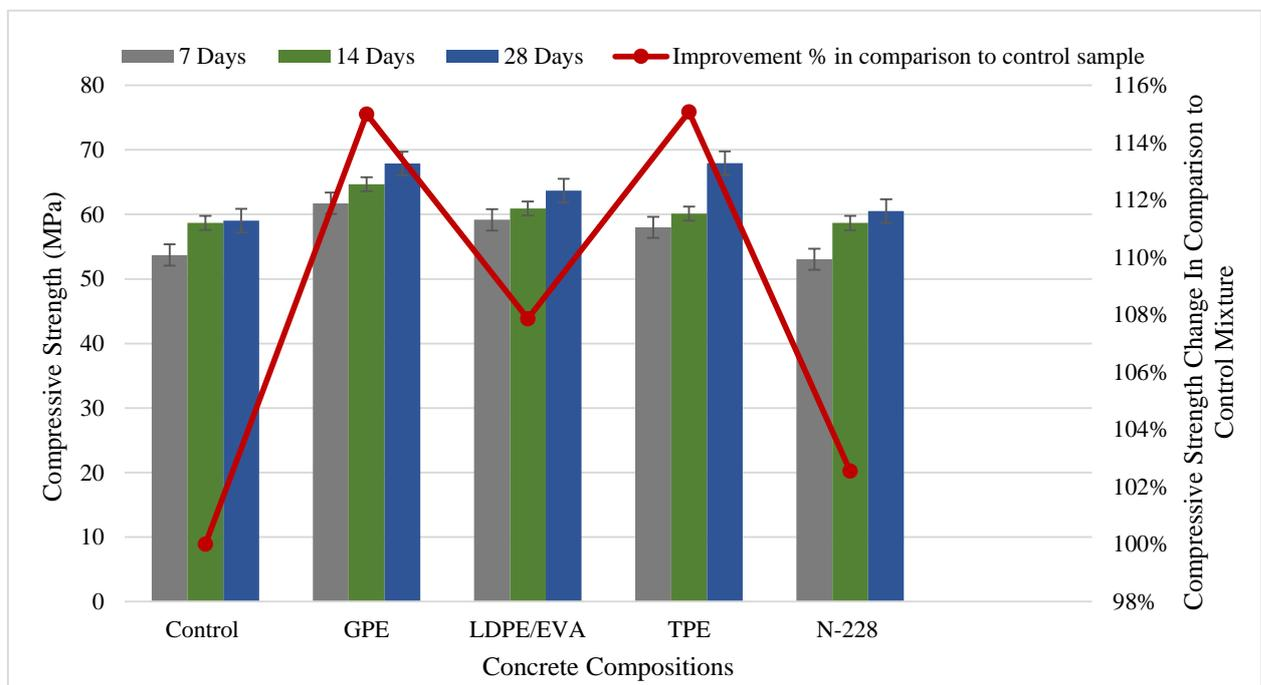
Figure 14 – Fine aggregate replacement by 3% powder thermoplastic polymer.
