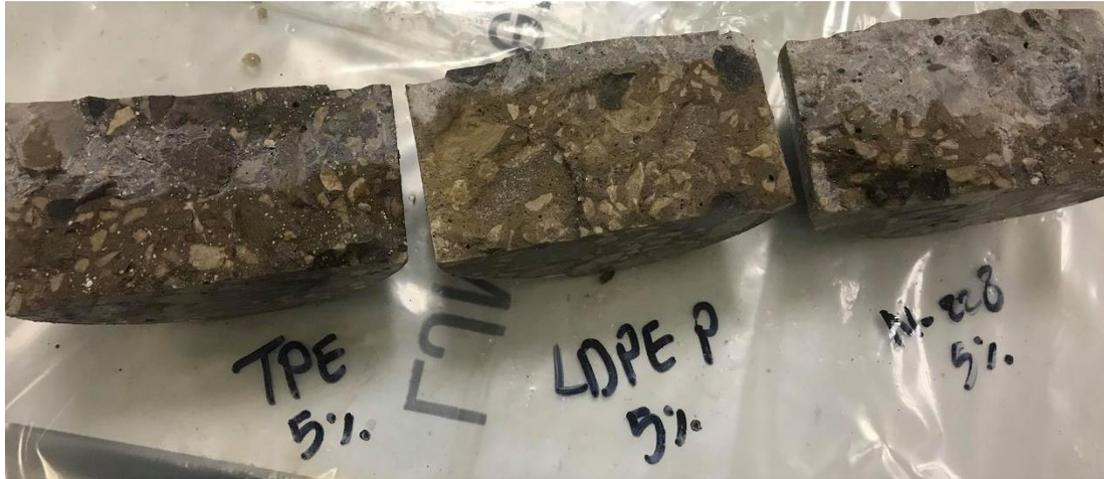
**Figure 21** – Chloride penetration in the concrete samples after 24 hours.
