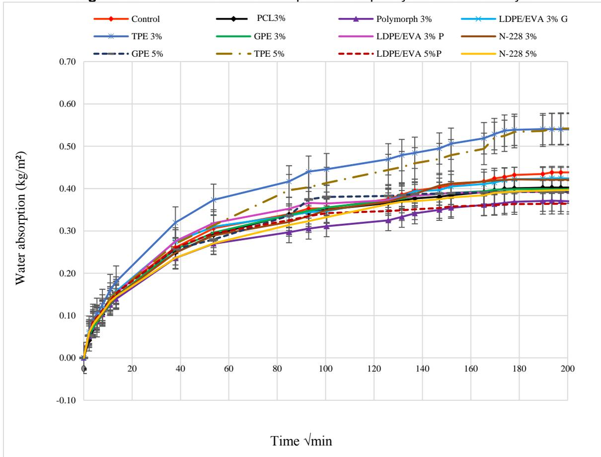
Figure 17 – Concrete water absorption via capillary for 28 days of duration.
