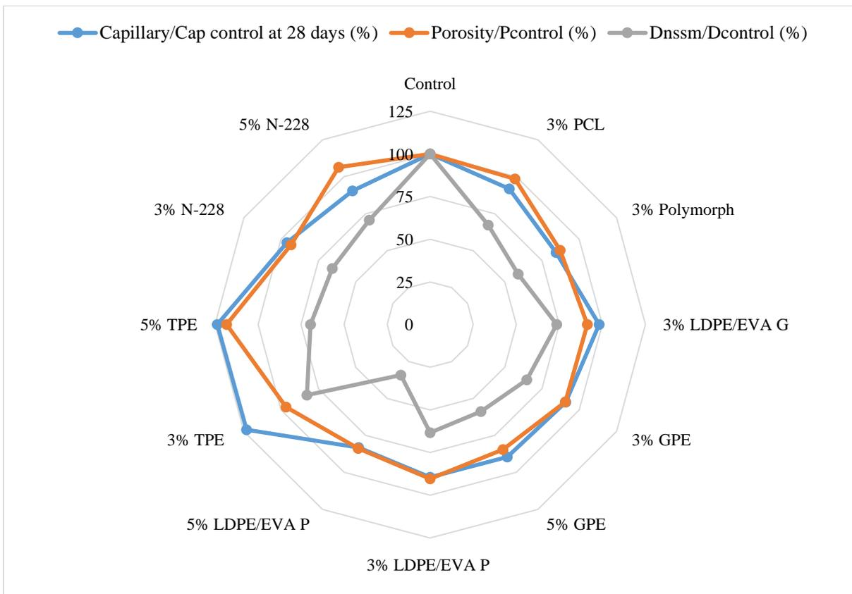
**Figure 22 – Impact of the use of polymers in concrete in comparison to OPC at 28 days.**
