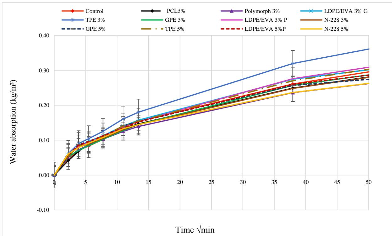
Figure 16 – Concrete water absorption via capillary for the first 2 days.
