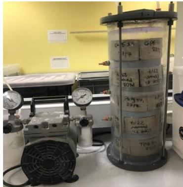
Figure 8 – Concrete open porosity test.
