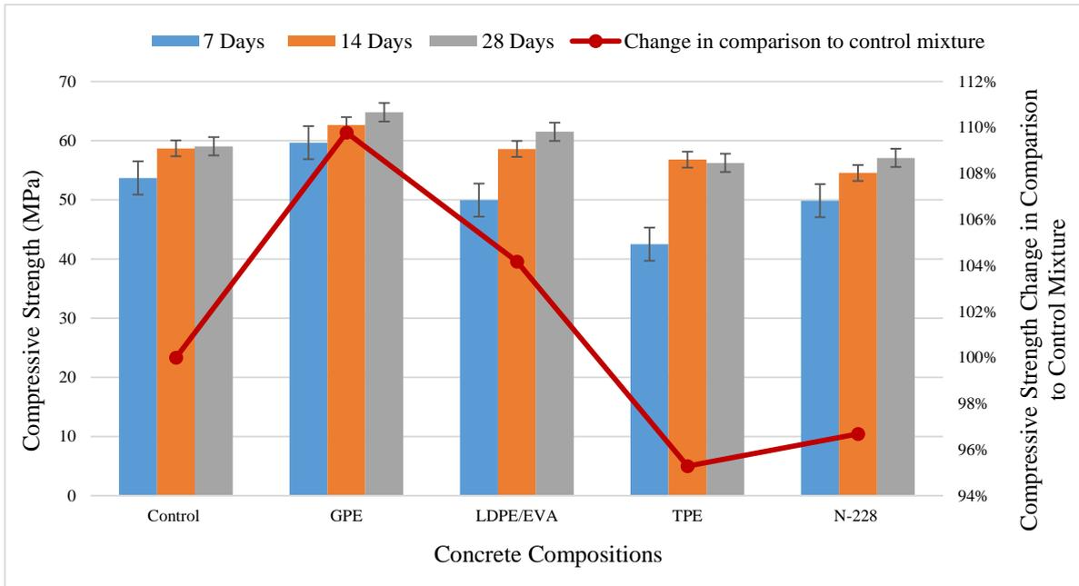
Figure 15 – Fine aggregate replacement by 5% powder thermoplastic polymer
