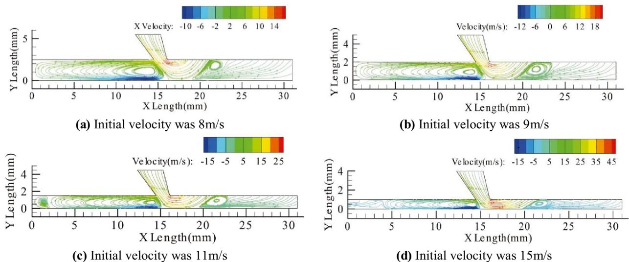
Fig. 6 The speed streamline of the abrasive jet flow in polishing zone
