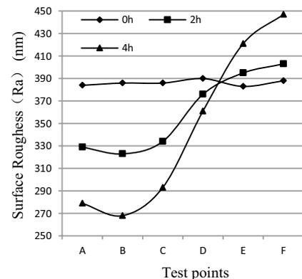
(b) The experimental surface roughness at different test points
