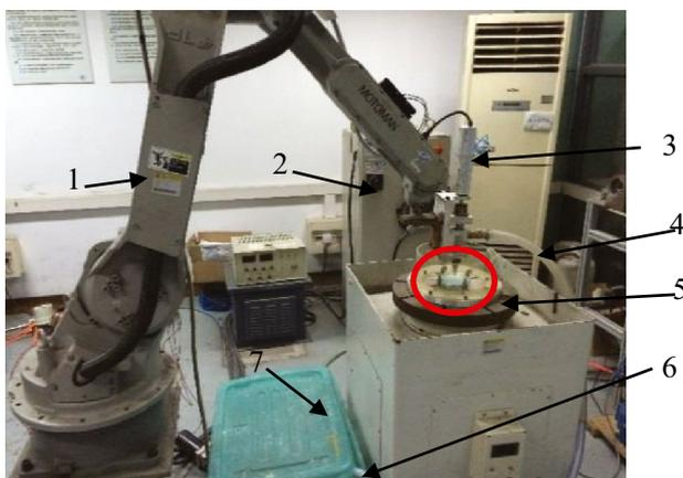
**(a)** Apparatus setup for AJP process
