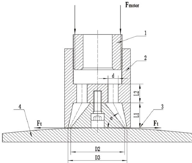
1 Nozzle, 2 shroud, 3 jet, 4 workpiece
