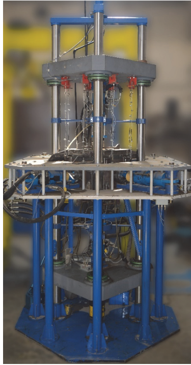
Figure 1. True triaxial testing apparatus: (a) Photograph, (b) Design drawing
