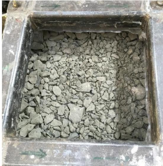
Figure 12. Subballast surface (Setup B)
