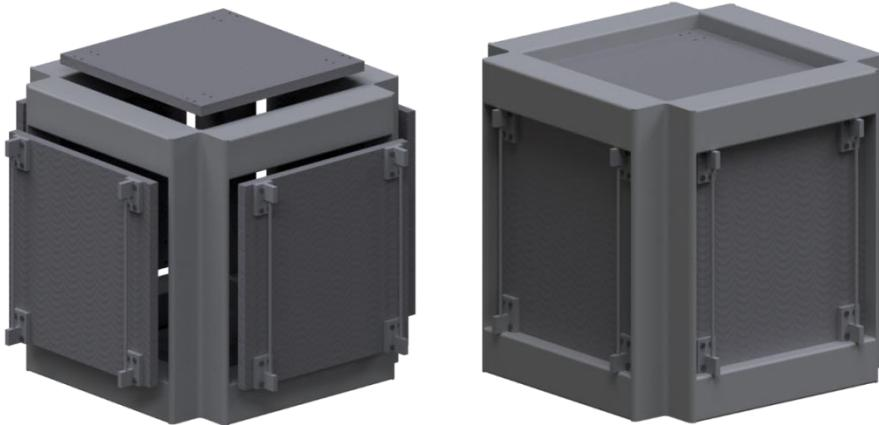
Figure 2. GeoTT testing cage: (left) walls contracted, (right) walls compressed
