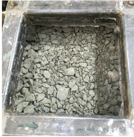
Figure 12. Subballast surface (Setup B)
