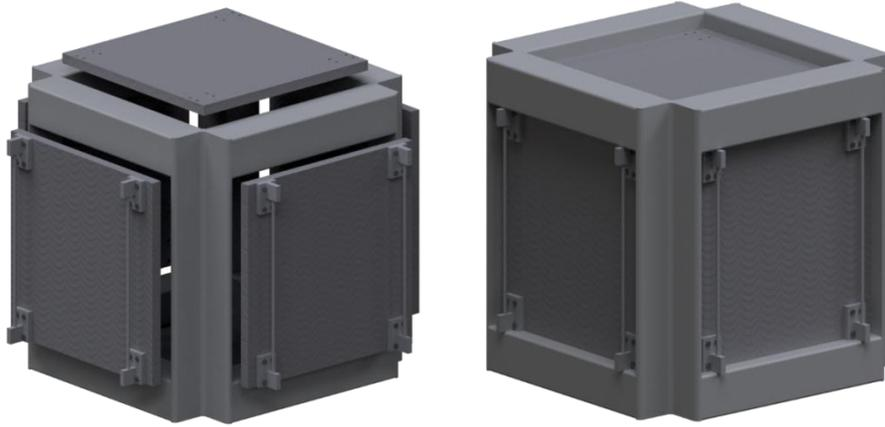
Figure 2. GeotTT testing cage: (left) walls contracted, (right) walls compressed
