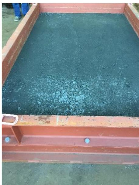
Figure 6. 400mm height of subballast
