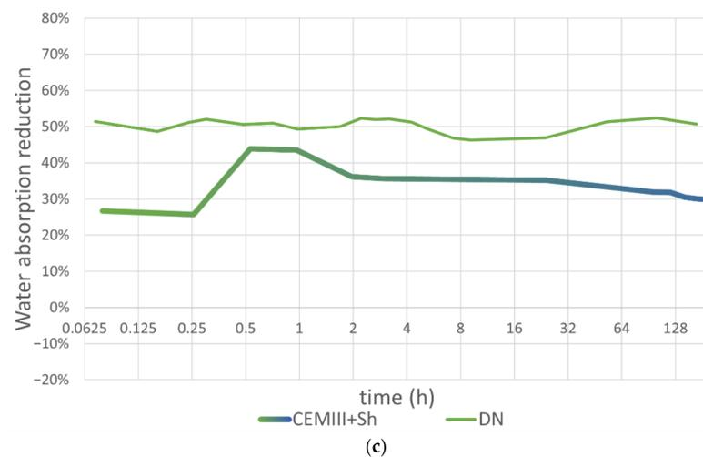
**Figure 8.** Comparison of water absorption reductions after treatment with selected repair or self-healing solutions: (a) “Intermittently wetted” solutions: VDB solution [46], M4 [63]; (b) “Constantly wetted” solutions: C1E5 [64], M2 [63], J solution [43]; (c) “Universal” solutions: CEMIII+Sh [65]; DN [66]. Colour code: green—bio-based; blue—inorganic based; solid line—internal solution; dashed line—external solution.
