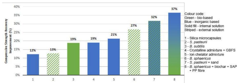
**Figure 5.** Improvement of compressive strength recovery of certain self-healing and crack repair solutions relative to unassisted recovery processes: 1—[4] (blank is the mix with less admixture); 2—[46]; 3—[59]; 4—[21]; 5—[20]; 6—[43]; 7—[47]; 8—[42].
