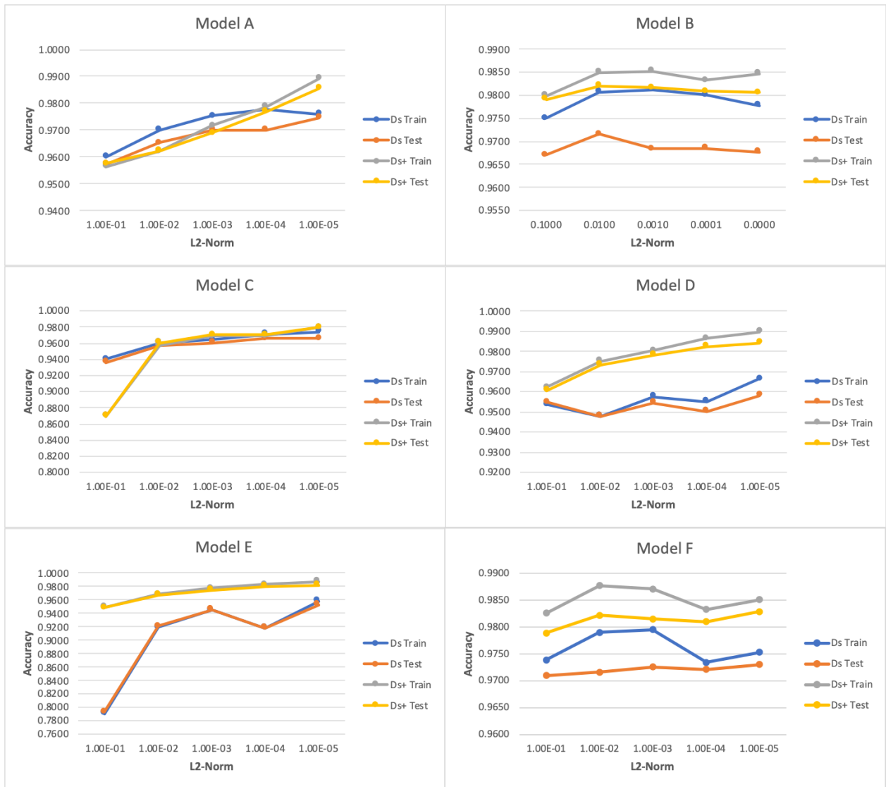
Fig. 4 Graphical representation of accuracy obtained from the CNN models trained on D_S^{tr} , D_{S+}^{tr} , and tested D_S^{ts} , D_{S+}^{ts} .
