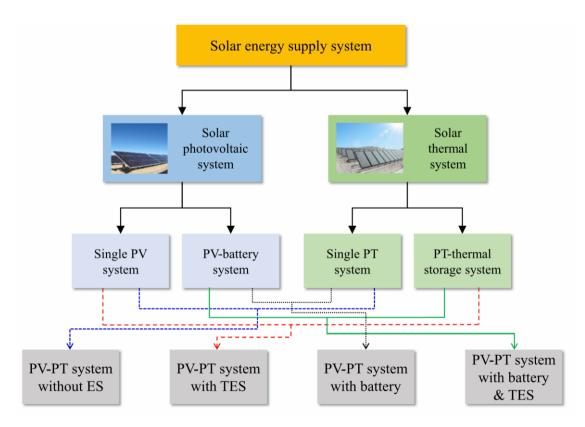
Fig. 3. Solar energy supply system for PSSBs.
