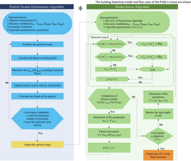
Fig. 5. Optimization model solving logic diagram.
