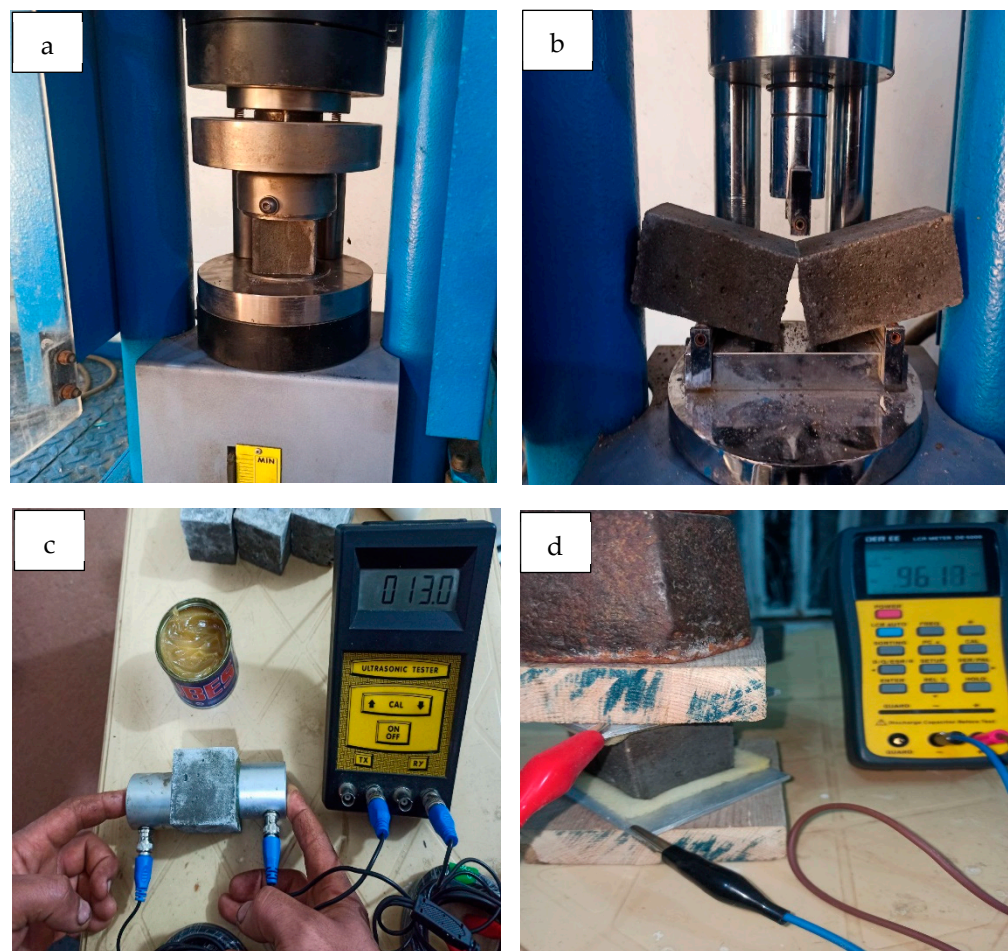
Figure 4. Some images of the experimental tests: (a) compressive strength, (b) flexural strength, (c) UPV and (d) electrical resistivity.
