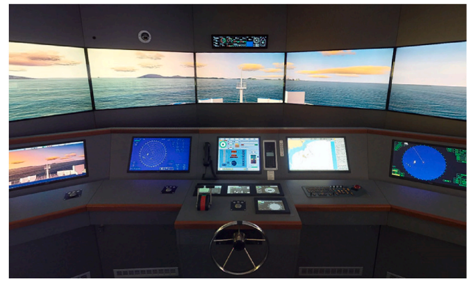
Fig. 3. The ship bridge simulator (Source: the authors).
