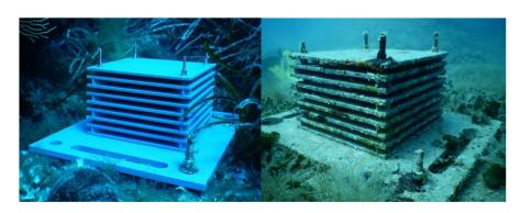
FIGURE 1 Autonomous reef monitoring structures (ARMS) during deployment (left) and a year later (right). Photos by Gabriele Giacalone.
