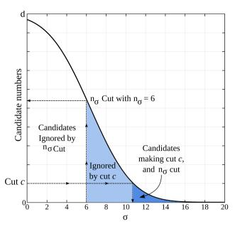
**Figure 2.** Diagram of 1 - CDF of equation (1), showing the relationship between  $n\sigma$  and constant cuts. This illustrates their impact on the number of noise candidates making it through to the candidate selection stage.
