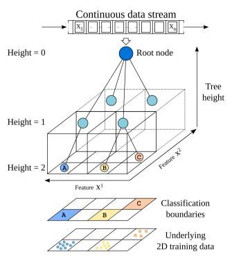
**Figure 7.** An overview of how a streaming decision tree partitions the data space to derive a classification. Each candidate is passed down the tree, and tested at each node it reaches including the root. Each node test outcome determines which branch the candidate continues down, until it reaches a leaf at the bottom of the tree. The tree shown here assigns the class labels A, B, and C to examples reaching the leaf nodes.
