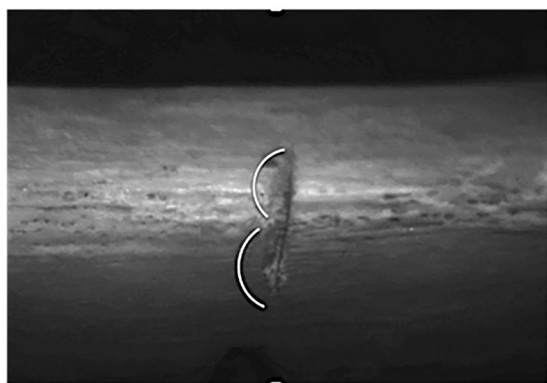
Figure 2. Example of grooves along the kerf wall.
