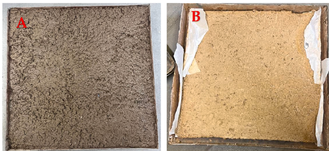
Fig. 1. A) Fresh cardboard paste, and B) Dried cardboard layer.
