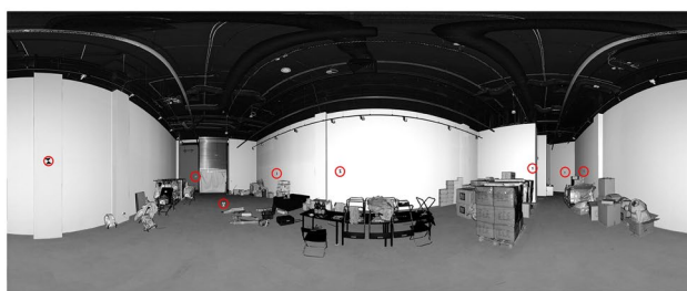
Fig. 8 The point cloud example in the spherical projection of test site VI with marked check points (red circles) [63]
