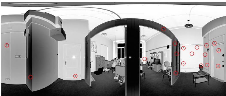
Fig. 7 The point cloud example in the spherical projection of Test Site V with marked check points (red circles) [63]
