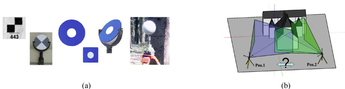
Fig. 1 a The example of the artificial targets, b registration between two scanned positions [27]
