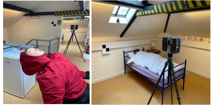
Fig. 3. 3D scanning at the crime scene facility after being adapted to simulate a crime incident.
