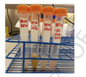
Fig. 14. Results for *beini*. Leftmost: blank solution; second from left: ferric chloride test; second from the right: Stiasny test; rightmost: lead acetate. The results show small amounts of tannins (photograph by the authors).
