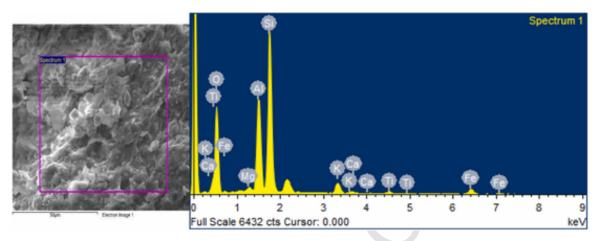
Fig. 19. SEM/EDS for plain mortar.
