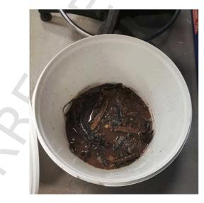
Fig. 10. Solution of dawadawa used for the earth-based mortars (photograph by the authors).
