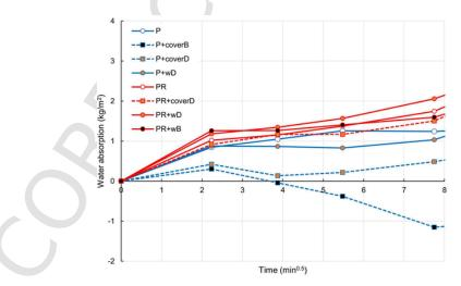
Fig. 17. Water absorption via capillary during the first hour.
