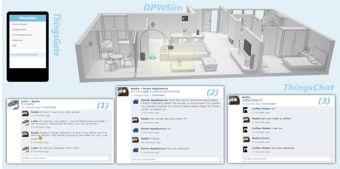
Figure 4. ThingsChat. ThingsGate is accessed by using smartphone via the mobile Web interface to discover and manage devices at virtual home of DPWS devices created in DPWSim. Below are different ways for the communication between people and devices. (i) There is a user Nadia sending Home Appliances group on ThingsChat to ask for receiving her mother Leila who is coming home while Nadia is still at the office. (ii) InRe accesses Nadia and Leila profile to recommend a list of services to be done at home, i.e., cleaning, opening the external gate, etc. (iii) Nadia accepts then most of the recommended tasks except the TV to be switched on. She also can directly chat with the coffee maker to prepare a coffee when her mother arrives.
