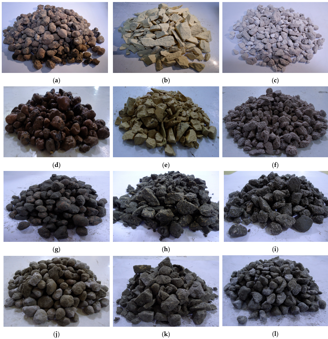
Figure 2. LWAs before and after treatment with various substances. SSD: Saturated surface dry. (a) Dry LECA; (b) dry CCB; (c) dry ACCA; (d) SSD LECA; (e) SSD CCB; (f) SSD ACCA; (g) pre-treated LECA with CG; (h) pre-treated CCB with CG; (i) pre-treated ACCA with CG; (j) pre-treated LECA with SFG; (k) pre-treated CCB with SFG; (l) pre-treated ACCA with SFG.
