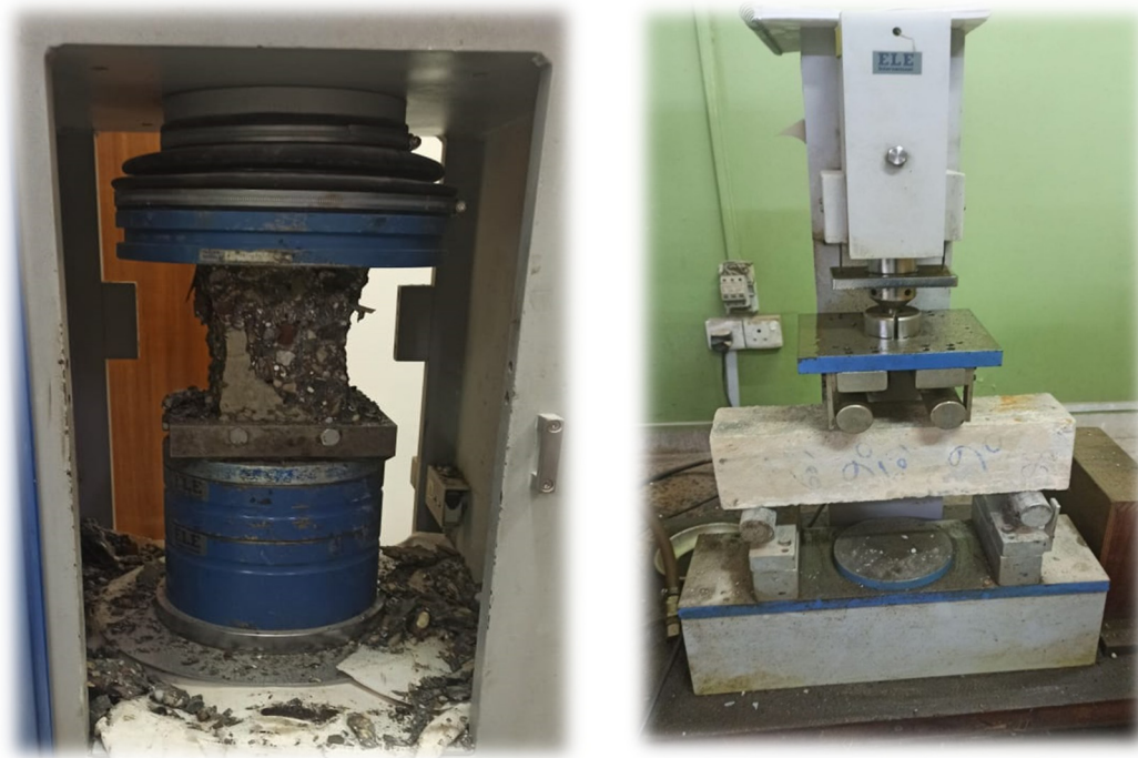
Figure 7: Samples under compressive strength test (left) and flexural strength test (right).
