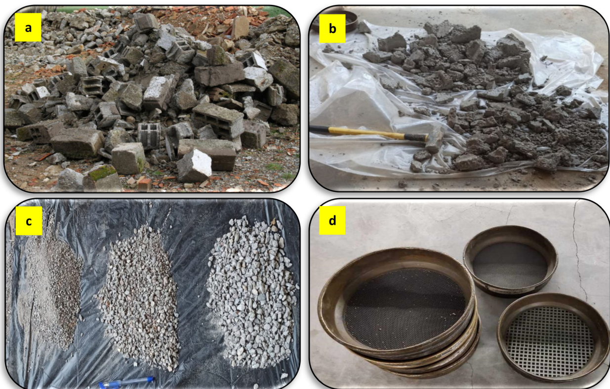
Figure 1: (a–d) Waste concrete block is recycled to create coarse aggregate (5–12 mm).
