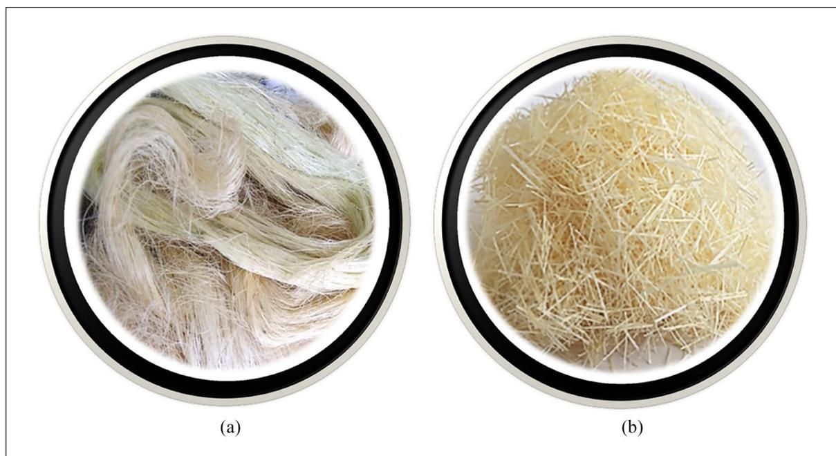
**Figure 3.** Raw AF employed in this study: (a) raw AF and (b) AF was cut into 19 mm length.
