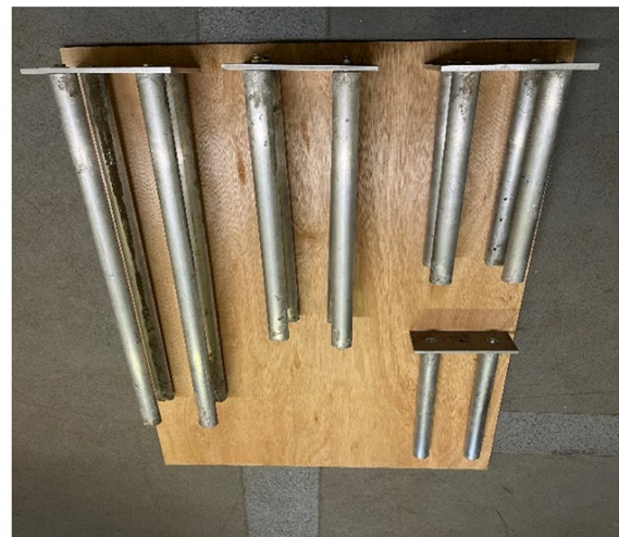
(b) CCFAT pile group models (2x2 and 1x2 configurations)
