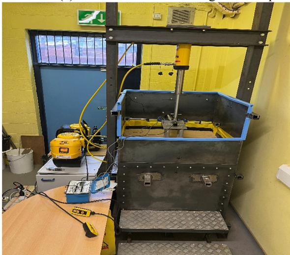
(b) Front view for testing CCFAT pile group 2x2 configuration
