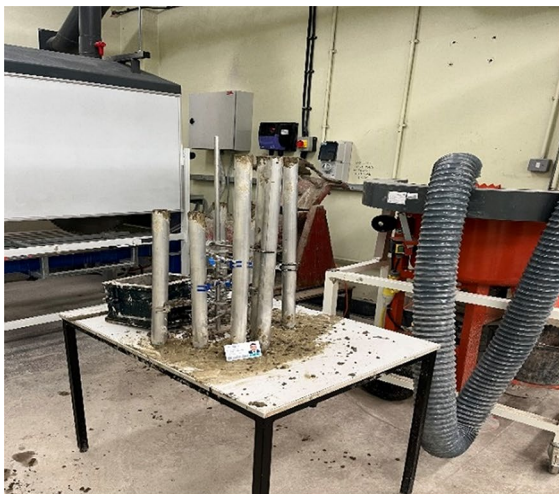
(a) Casting CCFAT pile specimens
