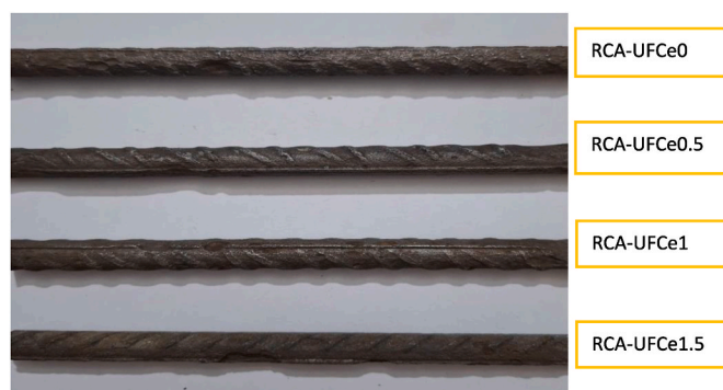
Fig. 18. Images of the steel rebars inserted into various RCA-UFCe concrete samples before sandblasting.
