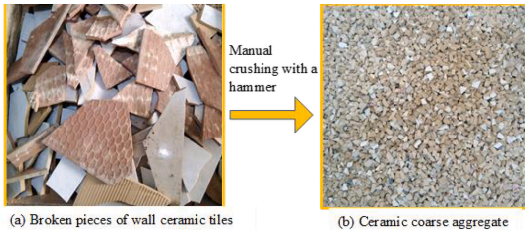
Fig. 2. The procedure for generating ceramic coarse aggregate from wall ceramic waste.
