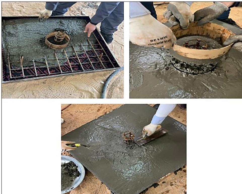
Figure 3. Specimen preparation and casting
