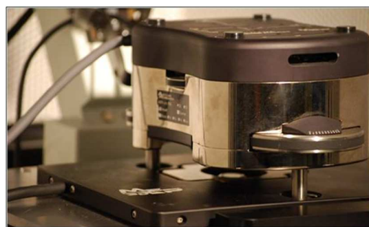
Fig. 1 Asylum research molecular force probe three-dimensional (3-D) atomic force microscope head that houses the optical lever detection system located above the microscope's sample chamber.
