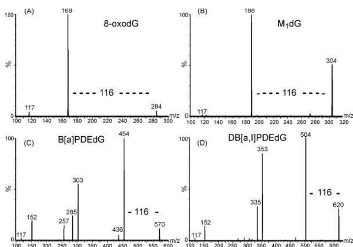
**Figure 2.** ESI MS/MS mass spectra documenting  $[M+H]^+$  to  $[M+H-116]^+$  transitions of four DNA different adducts; (A) 8-oxo-dG, the main oxidative stress related DNA adduct; (B) M1dG, the main malondialdehyde adduct; (C) B[a]PDEdG, the main benzo[a]pyrene diol epoxide DNA adduct; and (D)
