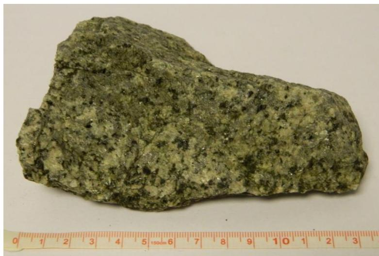
Figure 16: Photograph of sample 32 (site 15), Newry granite.
