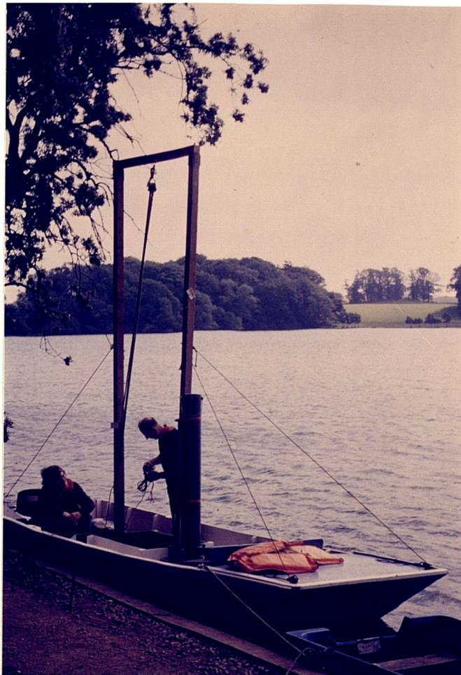
Plate 3. Ellesmere, showing the departmental 5m boat and gantry used to hold the 'Mini'corer vertical.
