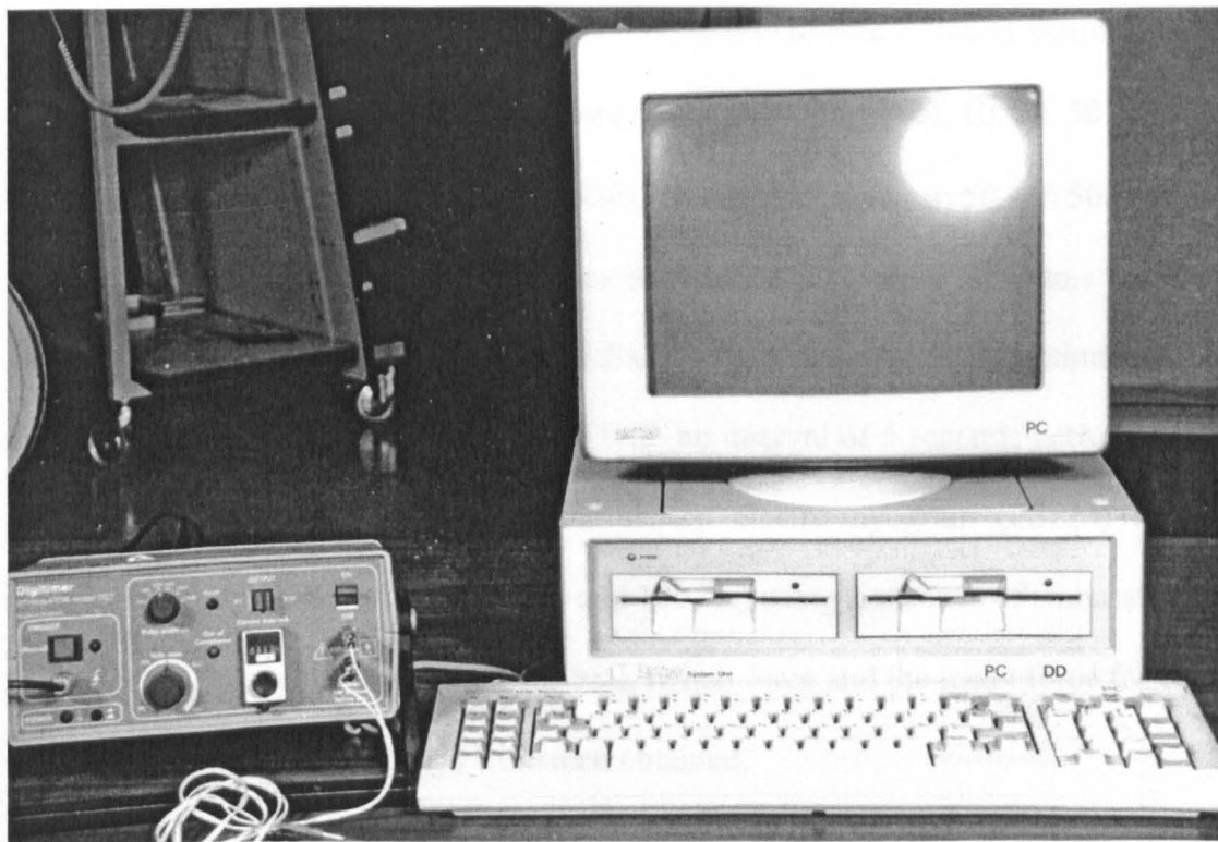
Plate 3.5 Digitimer high voltage stimulator driven by an Amstrad computer.
