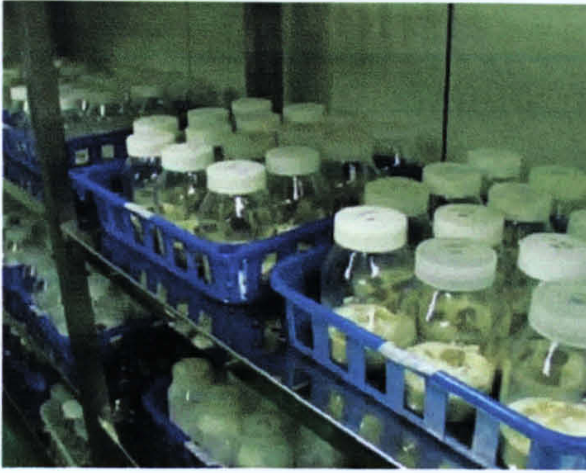
Fig. 2. 3. Sand culture vessels and wood block cultures inoculated with the test fungi.
