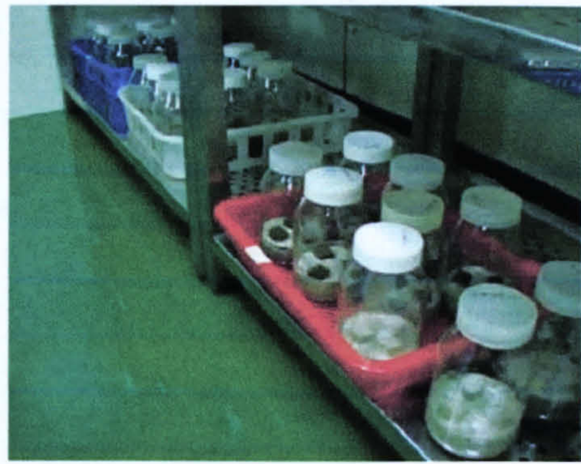
Fig. 2. 3. Sand culture vessels and wood block cultures inoculated with the test fungi.
