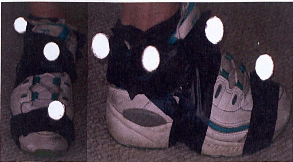
Figure 3.3 Foot tracking markers (front and side view)
