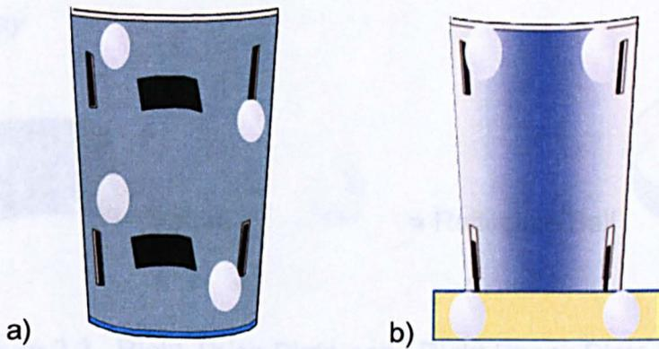
Figure 3.1 Trialled marker plates for shin, a) too small and ridged, b) wooden base (made to separate the markers as the plate wraps around the ankle) but plate too heavy. Markers size 25 mm (diameter).
