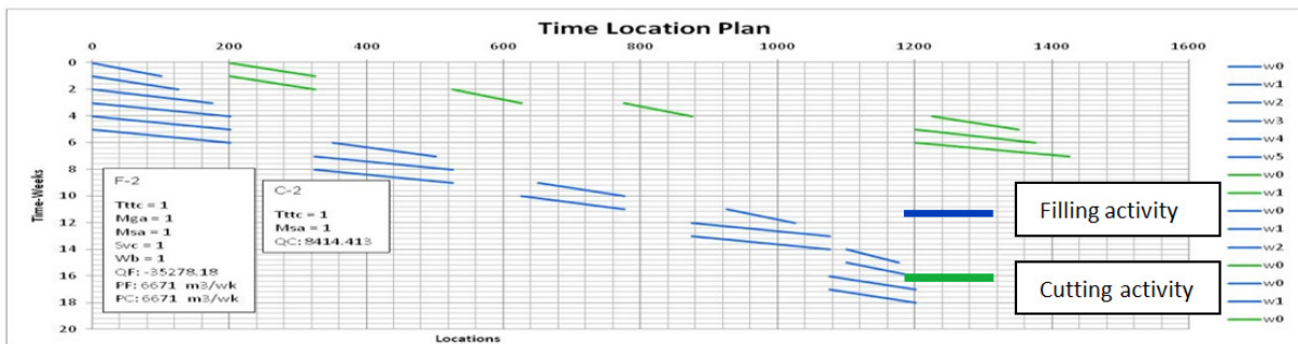
Fig. 4: Time-location plan of a road section generated by the prototype with option-1
