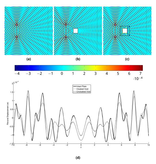
**Figure 6:** The flexural displacement generated by two coherent point sources in (a) an intact plate, (b) a plate with a square void, and (c) a plate with a cloaked square void. Figure (d) shows the interference fringes along an observation screen, indicated by dashed lines in figures (a)-(c). The following parameter values were used:  $\omega=100$ ,  $a=b=D^{(0)}=\mathrm{P}=h=1$ , and  $\epsilon=0.001$ .
