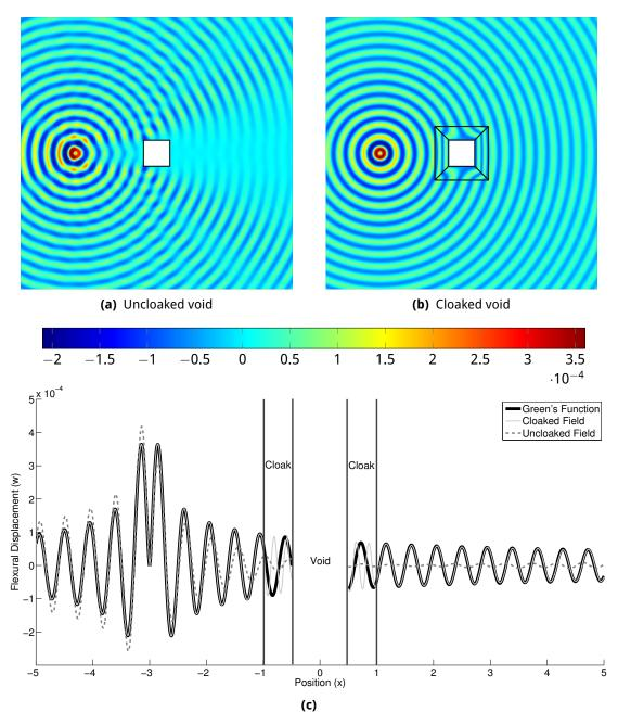
**Figure 3:** The flexural displacement w(x) generated by a point source in the presence of an uncloaked (a) and cloaked (b) void. Figure (c) shows the flexural displacement for cases (a) & (b) together with the Green's function for a Kirchhoff-Love plate along the line passing through the source and centre of the cloak. The non-dimensional radian frequency  $\omega=200$ .
