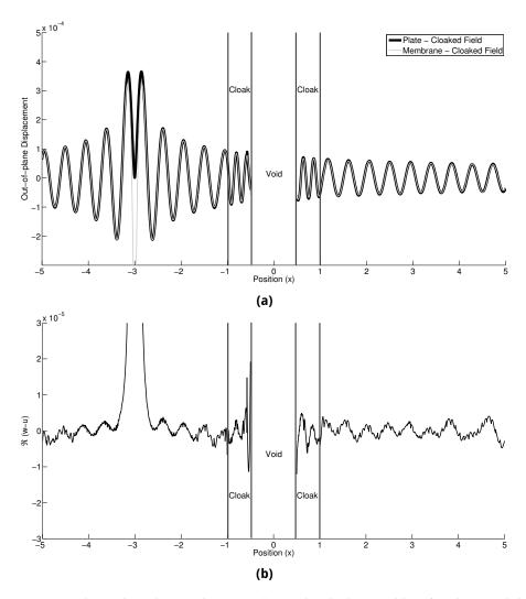
**Figure 5:** Figure (a) shows the solution when considering the cloaking problem for plates and the corresponding membrane problem. Figure (b) shows the difference between the solutions when considering the cloaking problem for plates and the corresponding membrane problem. In figures (a) & (b), the fields are plotted along the line passing through the source and centre of the cloak. The reader's attention is drawn to the different scales in figures (a) & (b).
