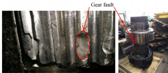
FIGURE 1. The faults of gear of the shearer ranging arm.
