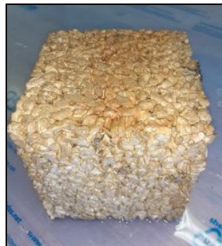
Figure 6. Precipitant formation across pervious concrete cube—column experiment.
