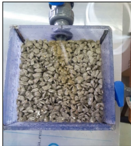
Figure 10. Precipitant formation across pervious concrete block—gravity experiment.
