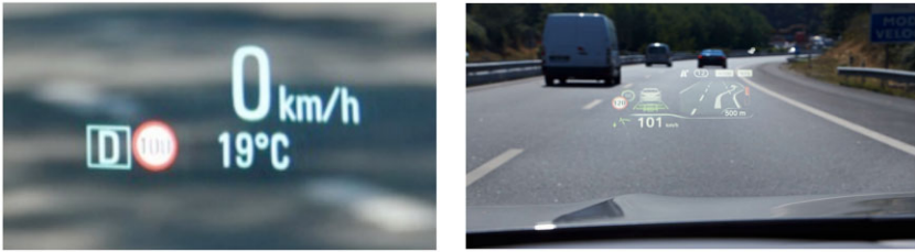
Figure 12: Heads Up Display (HUD) showing Speed Limit Sign Detection. Vauxhall (L) and BMW (R).
