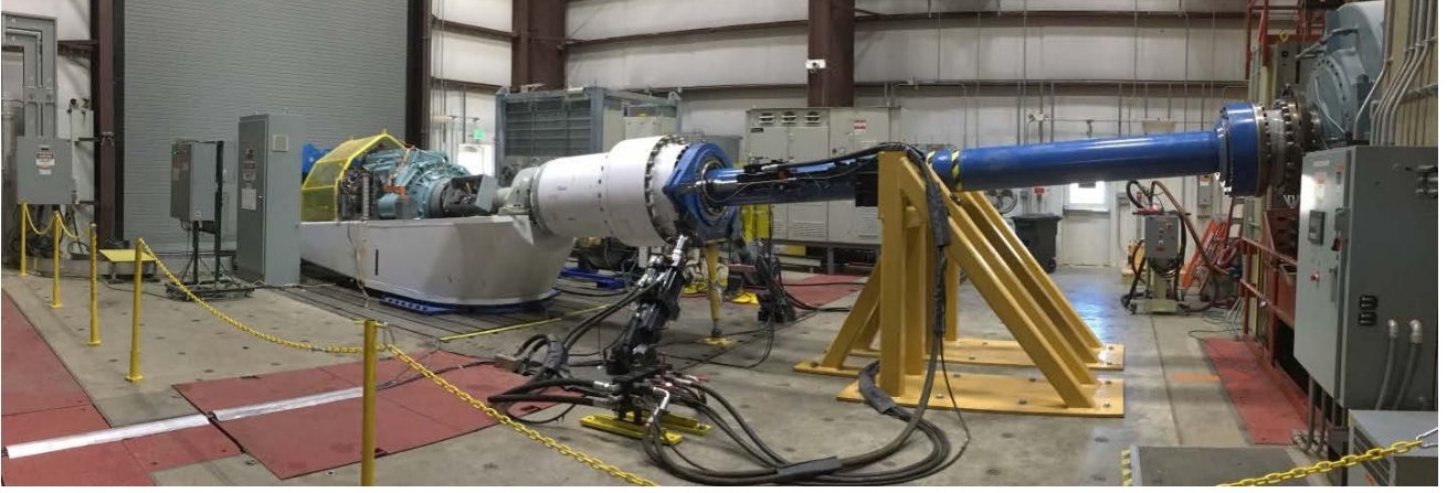
Figure 6: The real wind turbine drivetrain dynamometer installation
