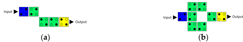
Figure 1. (a) Single-branch inverter. (b) Double-branch inverter. The blue colour indicates the input cell, the yellow colour indicates the output cell, and the green colour indicates the internal cells.
