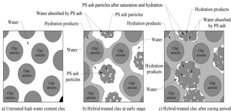
Fig. 6. The effectiveness of PSA in hybrid-treated soil [27].
