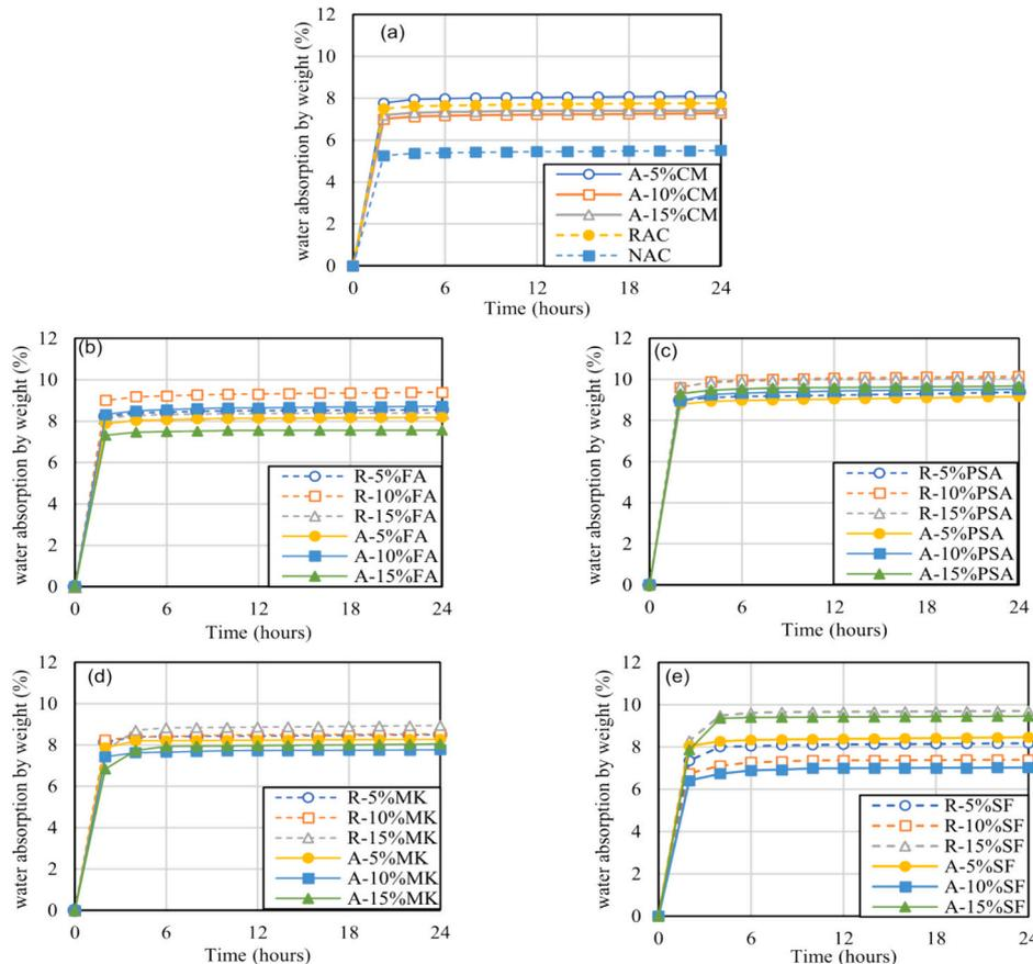
Fig. 4. Water absorption results [10].
