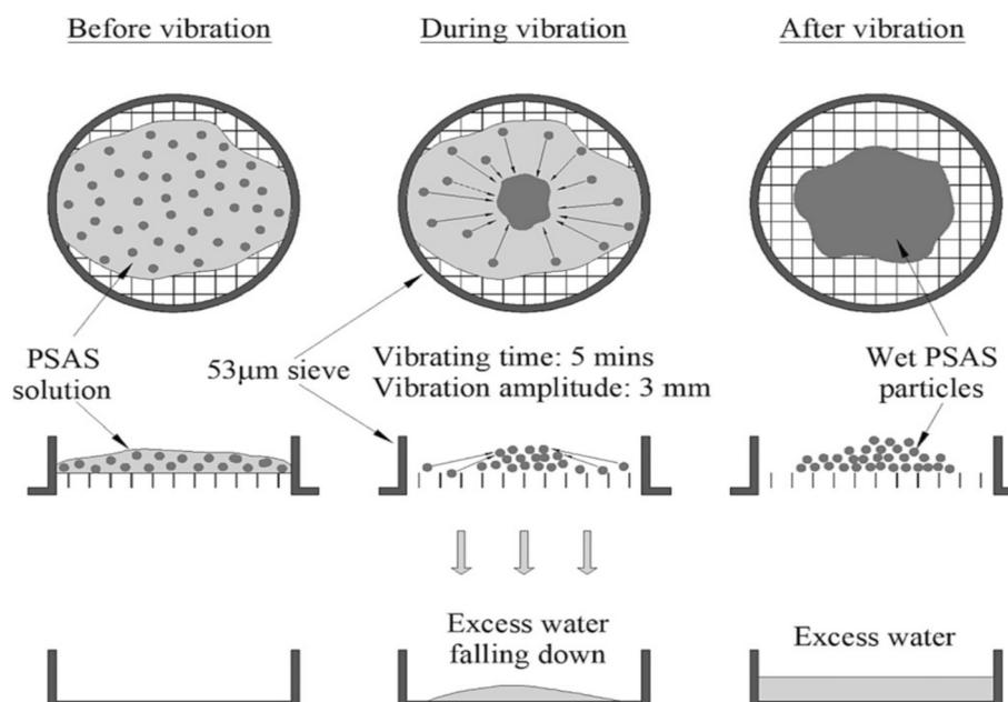
Fig. 5. Experimental principle for water retention and absorption rate of PSAS, Wab [27].
