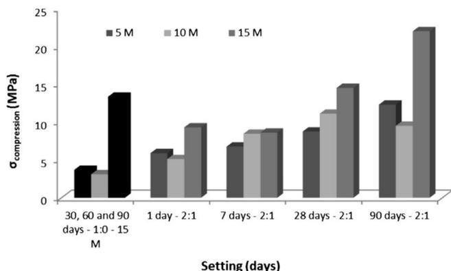
Fig. 9. Results for the compressive strength of geopolymeric samples made with an ash/calced paper sludge ratio of 2:1 [84].
