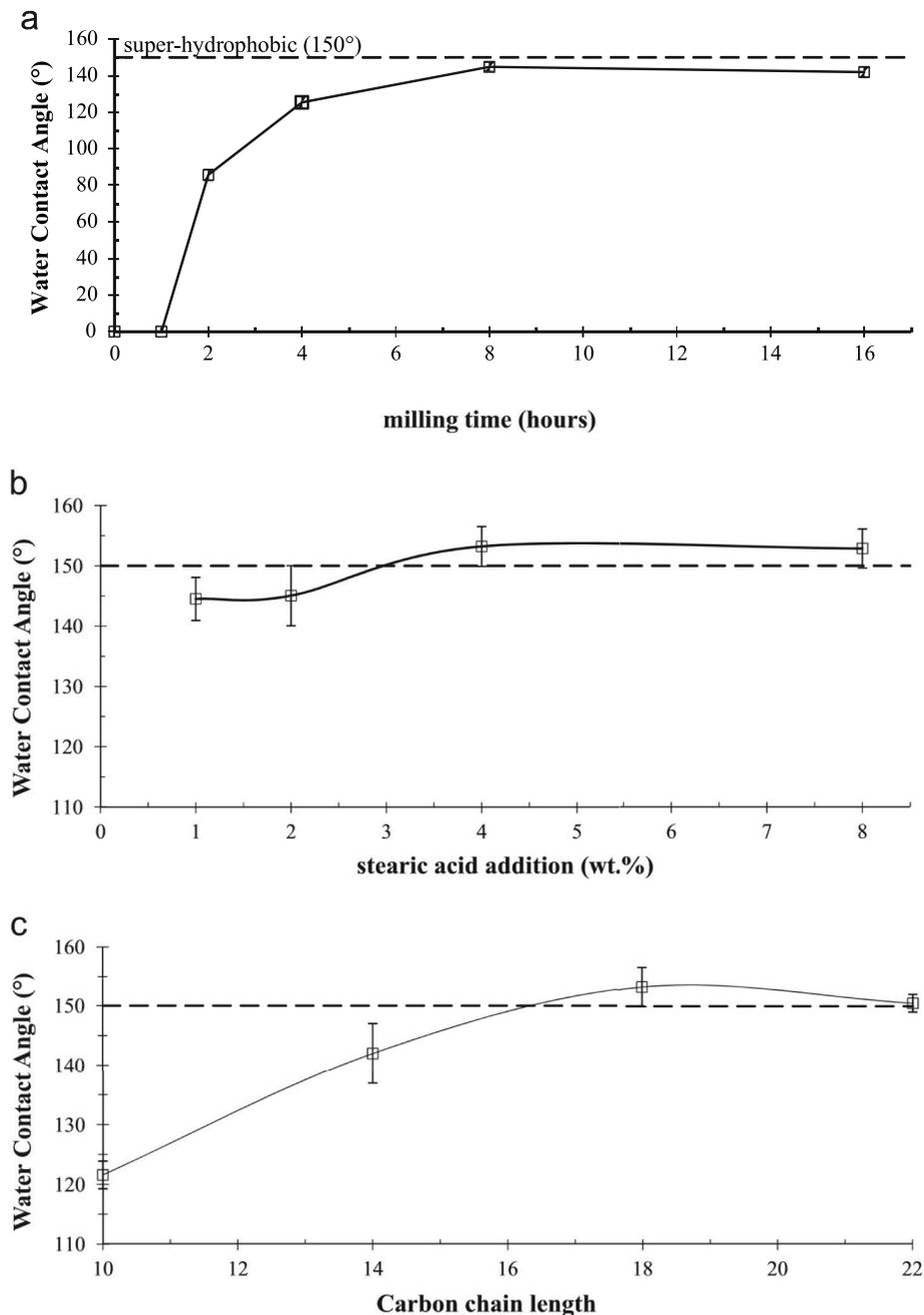
**Fig. 11.** Processing impact on PSA's WCA: A) the amount of stearic acid added at 1 wt% during the milling process, B) the amount of stearic acid dry milled for eight hours, and C) the use of various chain length fatty acids as surface functionalizing agents [32].
