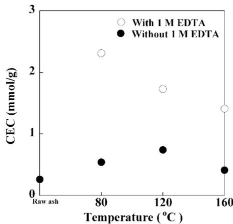
Fig. 10. CECs of PSA and the products produced from PSA at various temperatures with and without 1 M EDTA (3 M NaOH, 24 h of reaction time) [94].
