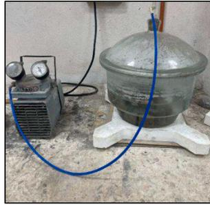
(b) permeable porosity test
