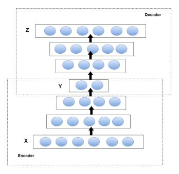
Figure 2. A deep autoencoder where intermediate layers provide increasingly more abstract representations of the input signal. The most abstract representation is stored in layer 4 (vector  $\mathbf{Y}$ ).
