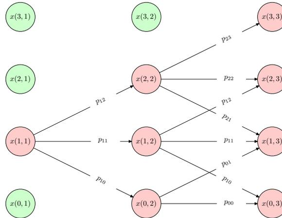
**Figure 3.** A spatio-temporal Markov chain for the processes of industrial production/service.  $P = \{p_{10}, \dots, p_{ij}, \dots\}$  ( $i, j \in \{0, 1, 2, 3\}$ ) is the set of processes,  $x(i, t)$  ( $i \in \{0, 1, 2, 3\}, t \in \{1, 2, 3\}$ ) denotes the state space at the time  $t$ , and  $i$  is the location number of the equipment that is with the state  $x(i, t)$ .
