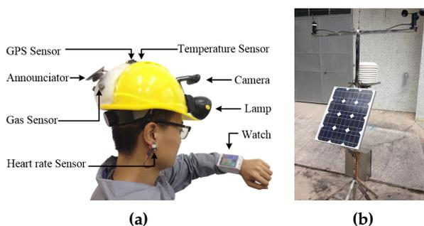
**Figure 5.** (a) Sensor-embedded wearable wireless devices: smart helmet and wrist watch. (b) Static wireless sensor node. The smart helmet is sensor-embedded, and it works with the wrist watch to dynamically detect toxic gases. The static node is supported by solar energy and enables to persistently measure the concentration of gases in the air, e.g., CO, SO<sub>2</sub> and CH<sub>4</sub>, and other environmental information, e.g., wind speed, humidity and temperature.
