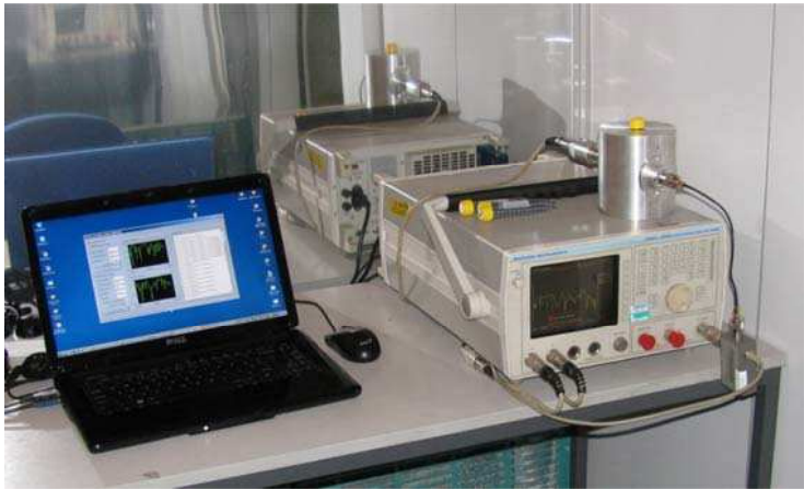
Figure 5. Experimental setup for the resonant cavity sensor.
