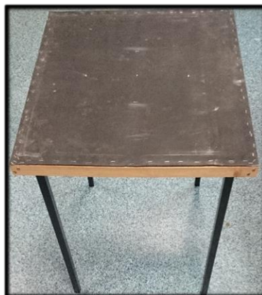
Figure 4: Concrete Paving Slab with a Membrane Layer
