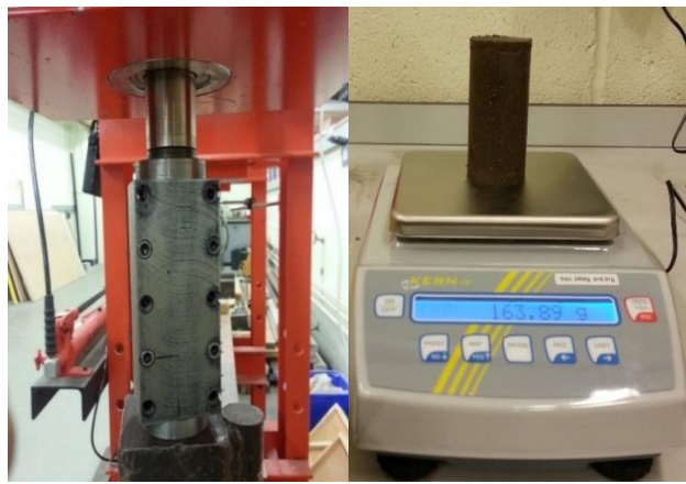
Figure 6: Hydraulic compaction and weighing of a specimen preparation
